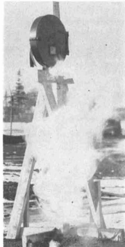
Fig. 4. Nitrate film during same simulated situation as in Fig. 3.
