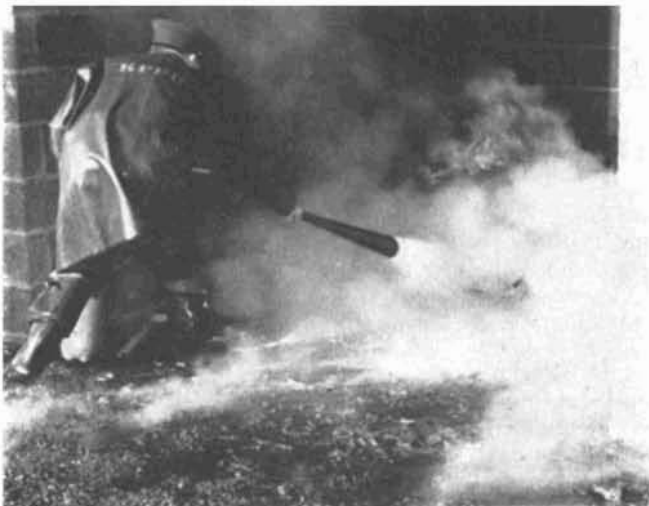
Fig. 7. Extinguishing acetate film in test fire.
