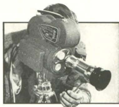
New professional turret of "Cine-Voice II" manufactured to highest precision standards and designed to take heavy-weight professional "C-Mount" lenses; can also mount zoom-type lens, as shown above.
