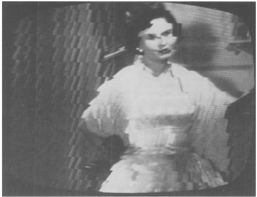
Fig. 2. Playback result when female guide is farther from drum than when recording was made.
