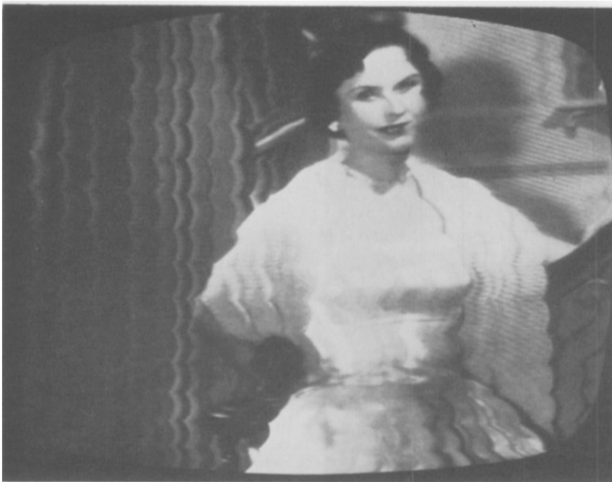
Fig. 7. Scalloping distortion resulting from vertical misadjustment of the guide.
