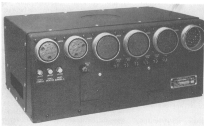
Fig. 2. Power supply unit for d-c power to operate the system.
