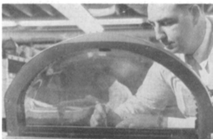
Fig. 5. "Windshield" model developed for integrated aircraft instrumentation.
