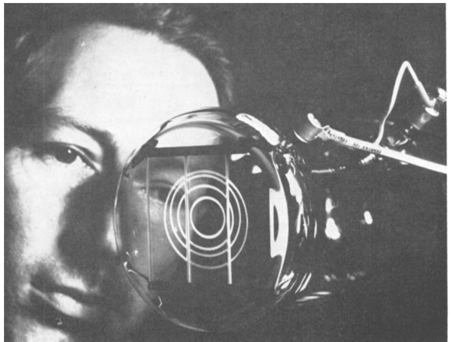
Fig. 1. The transparent cathode-ray screen
