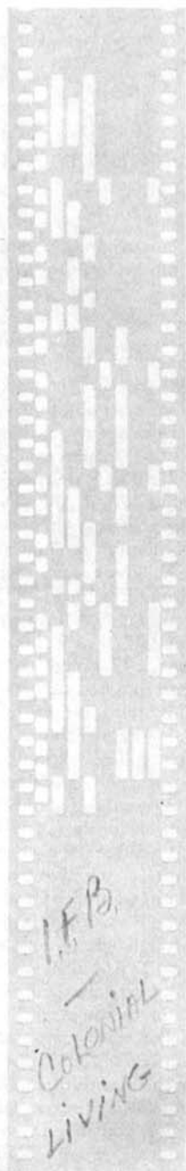
Fig. 7. Completed chart. First row on the left actuates fade-out and fade-in mechanism. The next three give various combinations of neutral density filters. The last four give various combinations of color correction filters.
