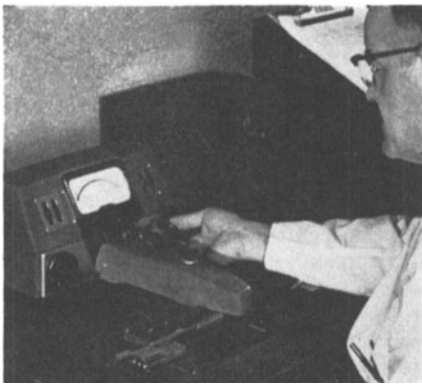
Fig. 5. Eastman Model 31A electronic densitometer used to measure processed strips.
