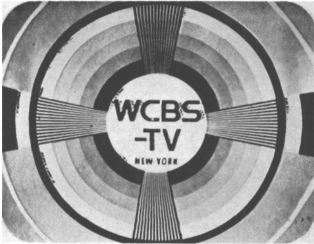
Fig. 10. Overdeviation: The carrier deviation produced by the leading transient overshoot of the white level signals are beyond the bandpass of the system and result in a streaked interference pattern following the transition from black to white.
