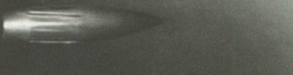
MICROFLASH This photograph made with newly developed EG&G Microflash (below). Light duration: .5 microsecond. Peak Light: 50 \times 10^4 horizontal candle power. Energy input: 8 w.s. (0.05 mfd @ 18 kv.). Plus-X, f/11. Price: $975.00 F.O.B. Boston. (Delivery from stock.)
