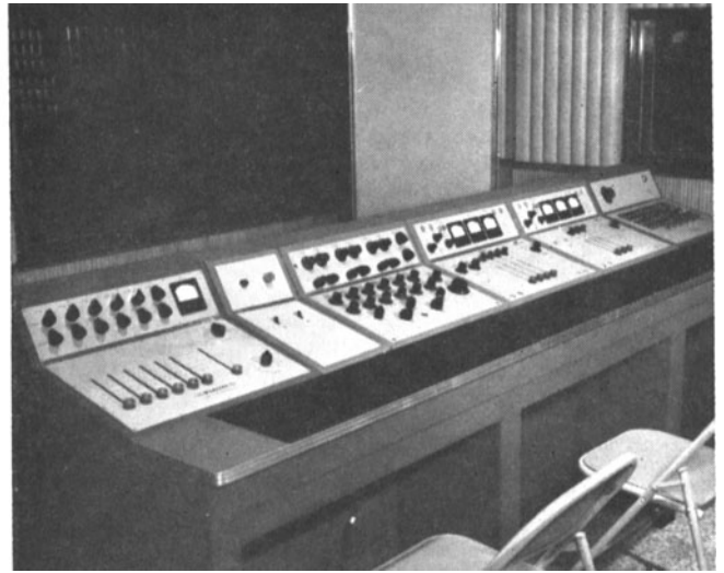
Fig. 2. Six-channel multitrack recording and mixing console. The two units on either end of the console as well as the console structure were fabricated in India.
