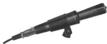
ALTEC 684A OMNIDIRECTIONAL MICROPHONE Frequency Response: 35 to 20,000 cycles • Output Impedance: 30/50, 150/250, 20,000 ohms • Output Level: -55 dbm/10 dynes/cm 2 • Hum: -120 db (Ref.: 10 -3 Gauss) Price: $78.00 net
