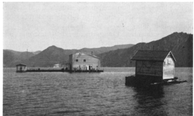
Fig. 2. U. S. Navy Electronics Laboratory calibration barge at Lake Pend Oreille, Bayview, Idaho, showing extension dock used to drape power and control cables into water. Small float in foreground holds transformers for boosting shore power to barge.
