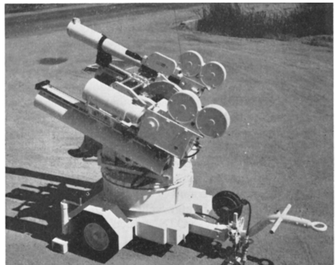
Fig. 6. M-45 tracking camera mount with 70mm, 35mm and 16mm high-speed cameras attached.
