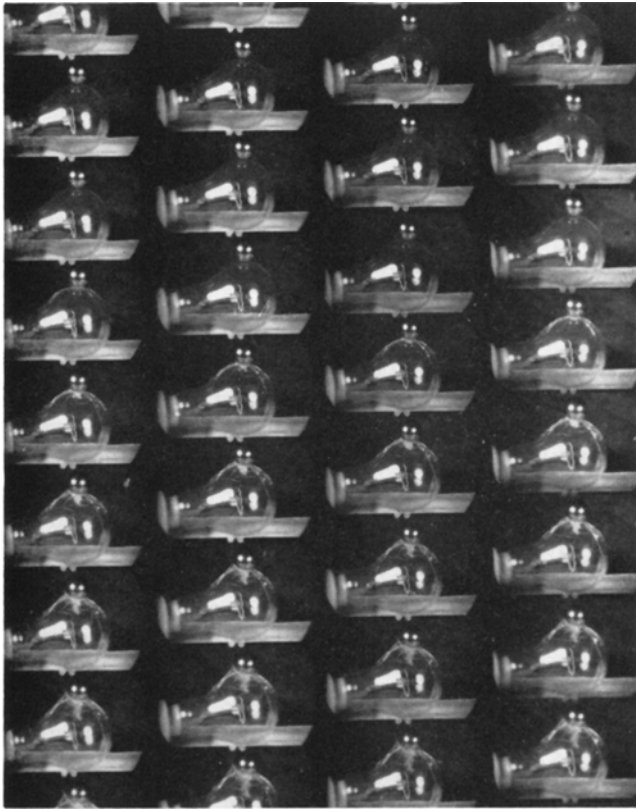
Fig. 12. A bulb being broken by a steel ball.
