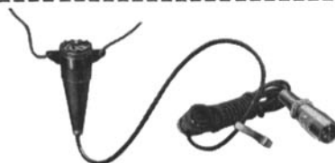
ALTEC 686A LAVALIER MICROPHONE Frequency Response: 70 to 20,000 cycles • Output Impedance: 30/50, 150/250 ohms • Output Level: -55 dbm/10 dynes/cm 2 • Hum: -120 db (Ref.: 10 -1 Gauss) Price: $54.00 net
