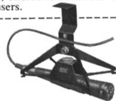
ALTEC 685A CARDIOID MICROPHONE SHOWN IN ALTEC 181A BOOM MOUNT Frequency Response: 40 to 16,000 cycles • Output Impedance: 30/50, 150/250, 20,000 ohms • Output Level: -54 dbm/10 dynes/cm 2 • Discrimination: Average front-to-back, 20 db • Hum: -120 db (Ref.: 10 -1 Gauss) Price $96.00 net
