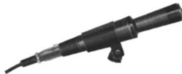
ALTEC 684A OMNIDIRECTIONAL MICROPHONE Frequency Response: 35 to 20,000 cycles • Output Impedance: 30/50, 150/250, 20,000 ohms • Output Level: -55 dbm/10 dynes/cm 2 • Hum: -120 db (Ref.: 10 -1 Gauss) Price: $81.00 net
