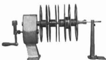
DFG-4 Differential Rewind to handle 4 reels
