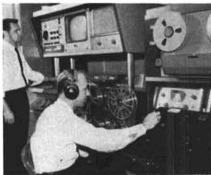
Fig. 2. Transfer of audio from video tape to 35mm magnetic film.
