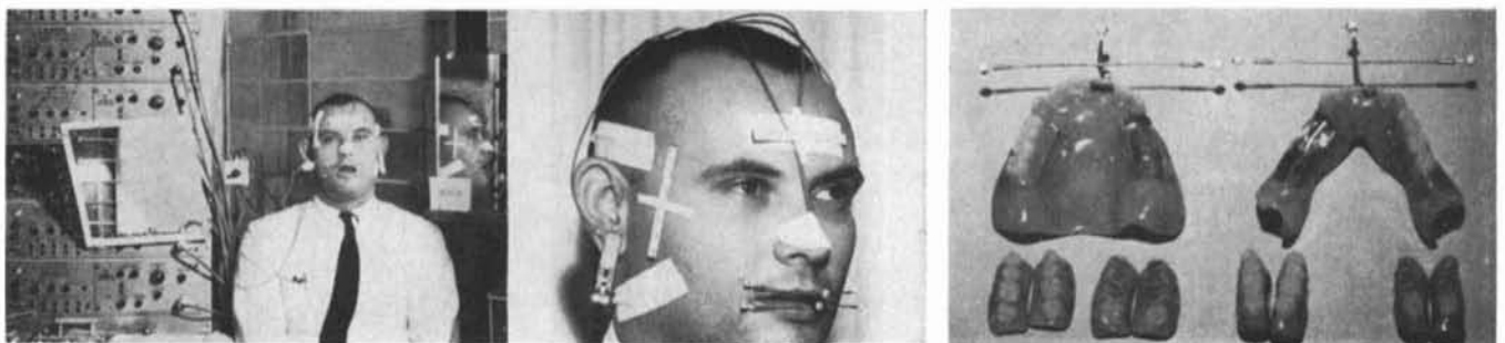
Fig. 1. Left: a Grass Model 5P3 Polygraph is used to record the activity of the muscles during jaw movements. Right: the movement of small white beads attached to the teeth with orthodontic bands is recorded on motion-picture film.
