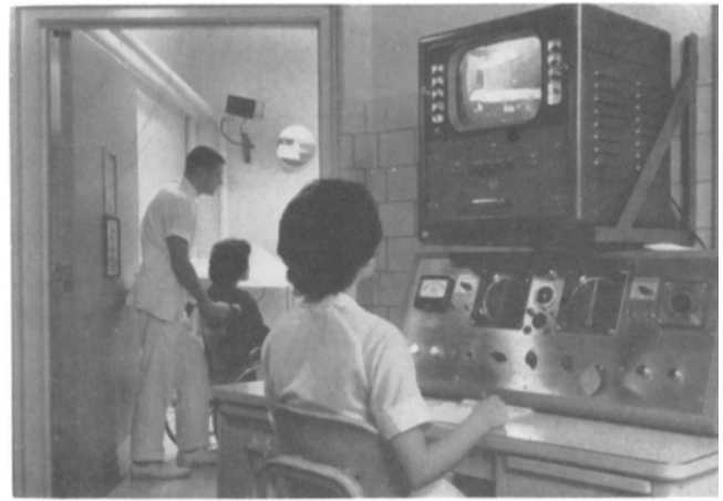
Fig. 5. One of three installations in Radiation Therapy Center at the Medical School. Vidicon camera, upper left, surveys patient under treatment and is monitored by technician.
