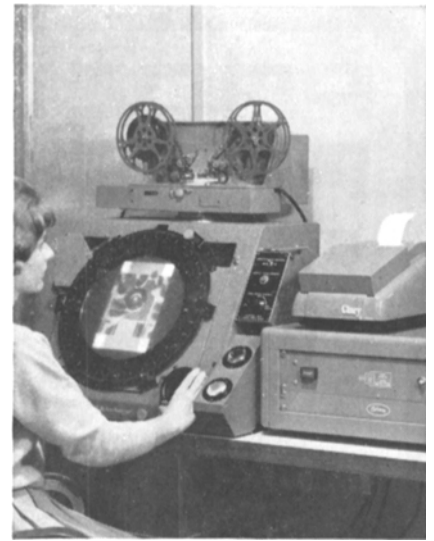
Vanguard Motion Analyzer shown with Coleman digitizing equipment and Clary printer. A wide choice of automatic readout/printout equipment is available to cut data-reduction time and improve accuracy.
