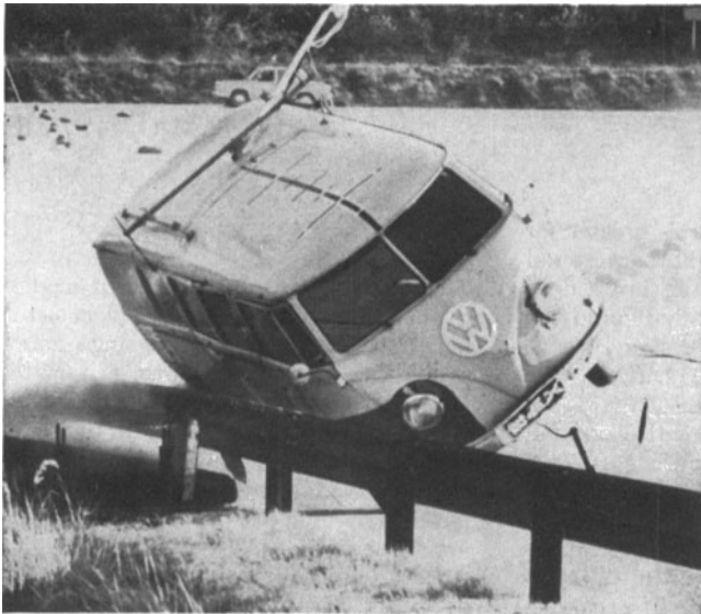
Fig. 3. Test collision between vehicle and test rail.
