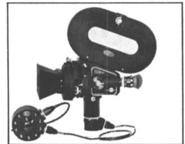
Arriflex 35 Model 2C-S. with all the features of the Model 2C, plus special 32 volt, DC motor, separate speed-control rheostat, and special tachometer, for operation to 80 fps
