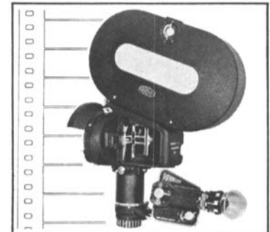
Arriflex 35 Model 2C-T. similar to Model 2C, but with movement for two-perforation pull-down and Techniscope film aperture (0.373" x 0.868"), 200° shutter and ground glass marked for Techniscope format. (Uses standard Arriflex 35 200 ft. and 400 ft. magazines.)
