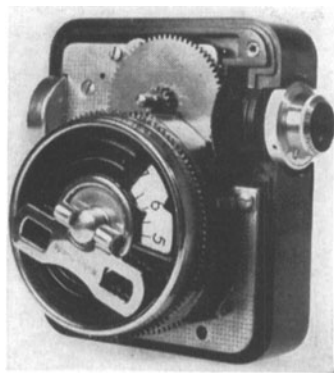
Fig. 1. Eumig C2, half of the housing (incorporating the viewfinder and the meter system) removed.
