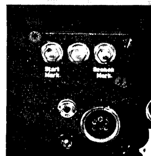
16BL rear view shows 60 cycle sync signal outlet, auto start marker and cue marker for double system.
