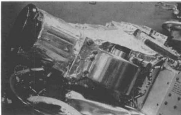
Fig. 15. Three-fourths front view of photographic system in lower half of pressure shell.
