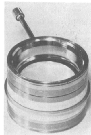
Fig. 3. Two-stage shutter tube image diameter of 35 mm.
