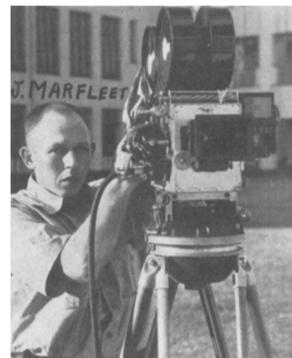
Fig. 2. Debie Model L camera rebuilt to handle 35mm films for bi-pack color; G. J. Marfleet behind camera.
