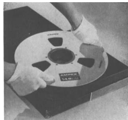
Fig. 3. Proper handling of magnetic tape includes lifting the reel of tape from its container by the hub and lower flange.
