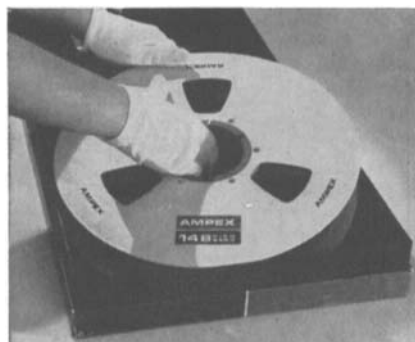
Fig. 3. Proper handling of magnetic tape includes lifting the reel of tape from its container by the hub and lower flange.
