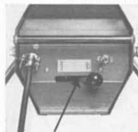
Full focusing controls for easy operation are shown in the LQTB-10 (motion picture model, above) and the LQTB-10/TV (television model, below).
