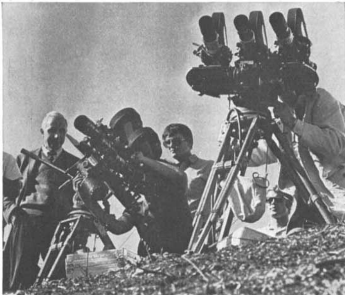
"US"—Another use of a triple Arriflex camera rig by Messrs. Thompson and Hammid, mounted on a common base that includes a belt drive so that one motor drives all three cameras synchronously. (PHOTO) Two separate triple Arriflex camera rigs are setup for filming of a location sequence.
