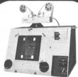
MOTION ANALYZER For X, Y, and Angle Measurements from Various Film Sizes
