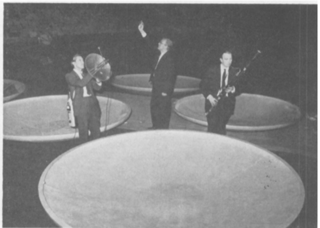
Fig. 2. Experts testing the acoustics — with bassoon music and a gunshot — while installing the “flying saucers.”
