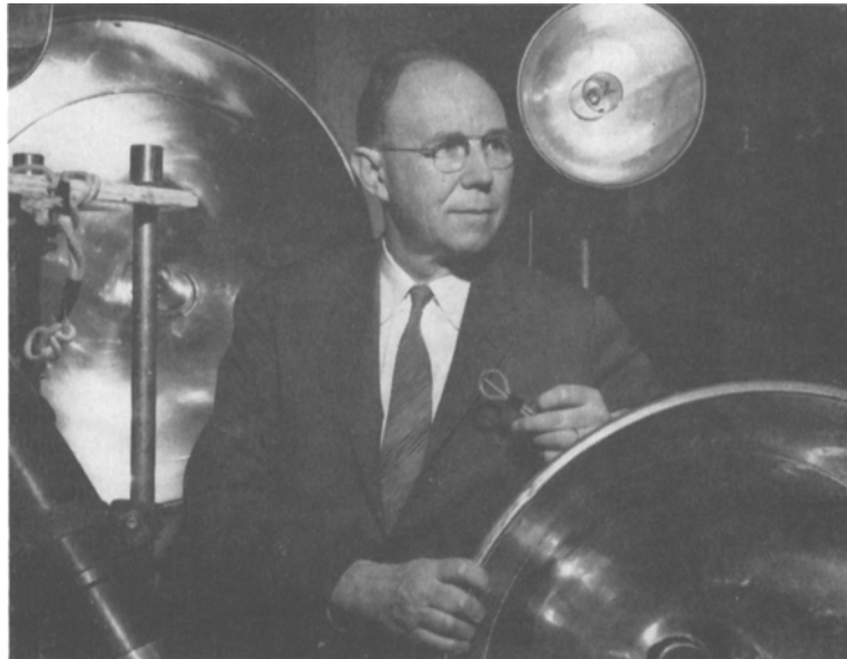
Strobe lights surround Prof. Harold Edgerton in his Strobe Lab at MIT. The large reflectors were used for aerial photography where 40,000-W/s were discharged into xenon flashlamps. He holds a small experimental flashlamp that has an exposure time of less than a microsecond. A descendant of this lamp is used for the photography of bullets in flight. Part of a deep-sea camera is shown at the left. The camera and strobe, designed for a depth of 36,000 ft, are at the Smithsonian Institution, Washington, D.C.
