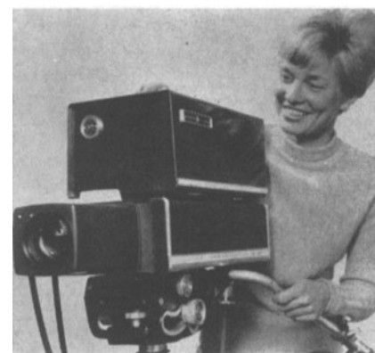
A 22-lb live color camera designated the TE-201 has been announced by General
