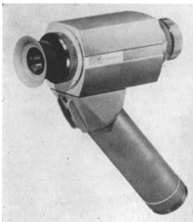
The Find-R-Scope, a handheld infrared viewer of the active type operating in the near infrared range has been an-
