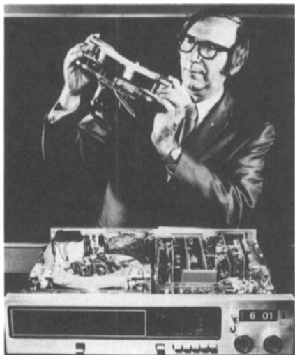
The SelectaVision MagTape player-recorder, designed as a self-contained package for use with an unmodified conven-
