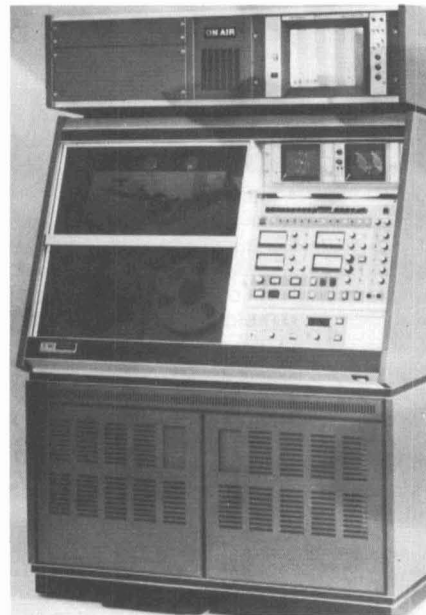
The IVC-9000, a broadcast videotape recorder using the helical scan format, de-
