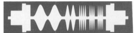
Fig. 7. Frequency response test chart: 400-Hz, 1-kHz, 3-kHz, 4-kHz and 5-kHz, modulated 80% with 50% unmodulated track.
