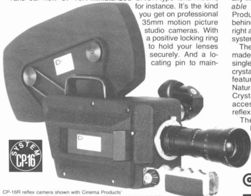
CP-16R reflex camera shown with Cinema Products' non-orientable viewfinder, with eyepiece located approximately 1" (25mm) behind the film plane; Angenieux 9.5-57mm zoom lens, with CP-mount; plus PLC-4 lightweight 400 ft. (122m) magazine, made of glass-filled Lexan®
