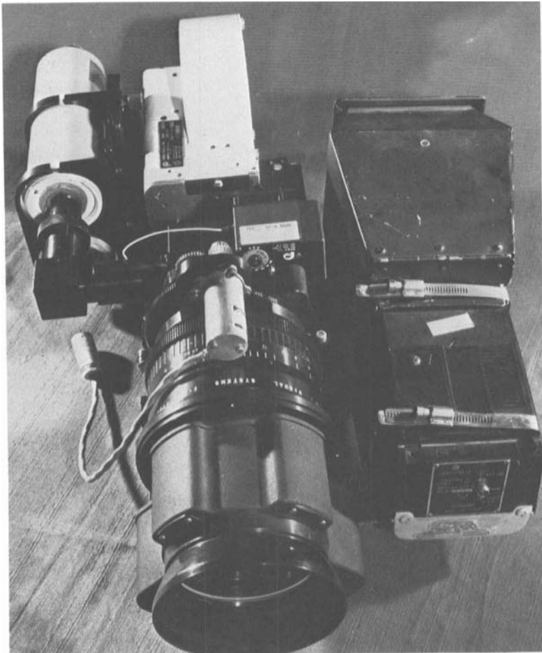
Fig. 6. The completely redesigned Photosonics camera system with the video monitor on the magazine side of the camera (r).
