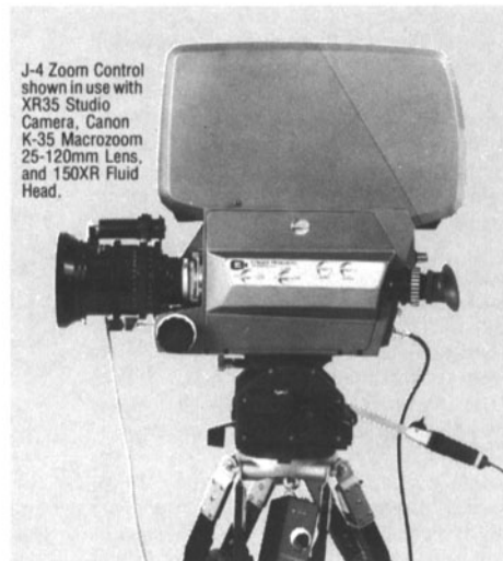
J-4 Zoom Control (zoom motor, compact zoom speed control box with built-in rechargeable nickel cadmium battery, battery trickle charger and "Joy Stick" control)
