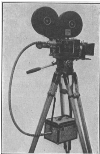
FIG. 2. Audio-Camex portable recording system attached to a camera.
