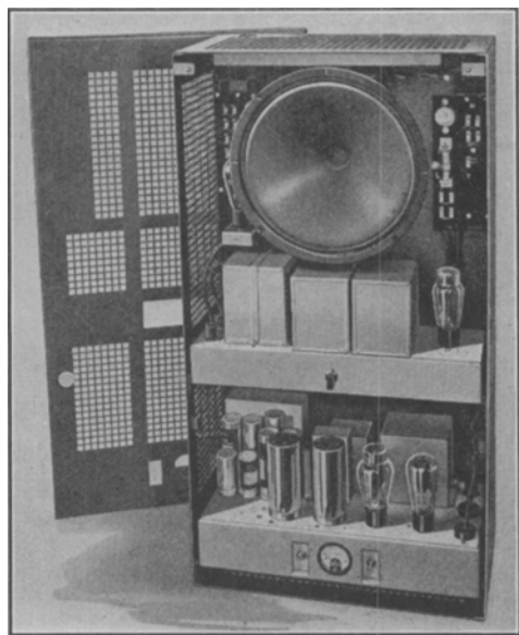
FIG. 6. The cabinet containing the amplifier, rectifier, monitoring loud speaker, and associated equipment.
