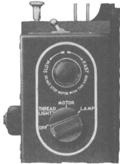
FIG. 4. Unit control for thread-light, motor, and lamp.
