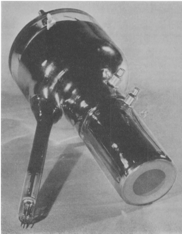
Fig. G. The Philips Image Iconoscope, Type 5854.
