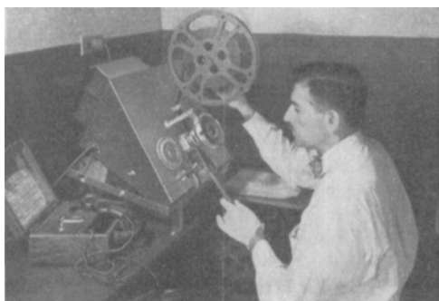
Only intelligence and skill can be depended on to select a timing value for correct printing. That's why a perfect print is a collection of scenes, each expertly timed.
