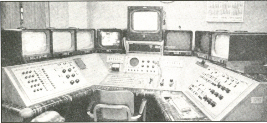
(Left) Control console with auto switching in Control Room 1; (Right) Remote-controlled camera • Automatic Switching at the Edmonton Television Studios • S. Glover • JSMPT E, November 1966.
