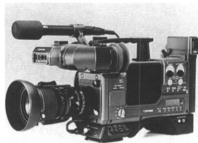
Toshiba America multiformat Hi8 3CCD camera/recorder
