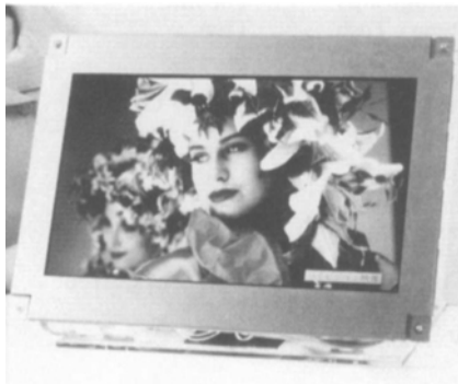
Sharp Corp. multimedia-compatible 16.5-in. color TFT LCD
